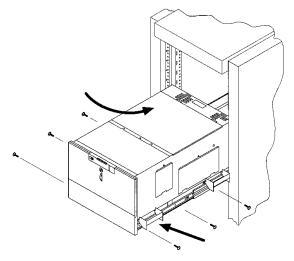
6. Remove the installation handles by removing two screws on each handle. Keep the screws and handles in case the library needs to be reshipped in the future.
